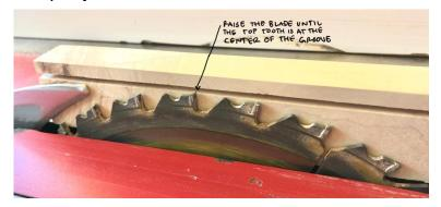
5. Now set your fence to the thickness you want the outside wall of the frame. In this case we will set the fence to 3/8". 3/8" should be the minimum for any frame larger than 8 %" x 11". Any thinner and problems could arise later in putting the frame together and preparing it to hang on the wall.
