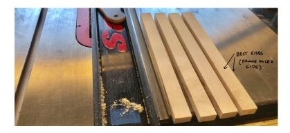
3. Set your table saw's fence to ¼" and using a feather board to keep the material against the fence run all 4 sides of your frame through the table saw. This cut WILL NOT cut all the way through the material but will make a groove.
