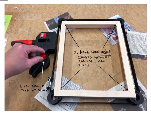
6. Twist the high tension handle to tighten twisting about two to three twists (not quite a half rotation for each twist). Recheck to make sure the inside corners match and the faces are flush. Don't worry about the back of the frame, only the front. Twist the high tension handle two to three more twists and recheck corners one last time.
