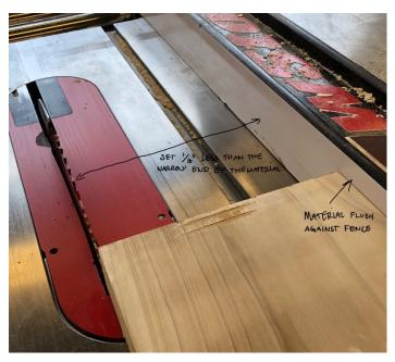
5. Flip your material and repeat the cut subtracting another 1/16" on the finish cut side. You should now have two clean parallel sides to your material.
