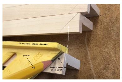
3. Set your miter saw to 45°. Before you make your cuts make sure your material is flat and tight against the base and back of the miter saw and that you are holding the material within the safe zone of the saw.
