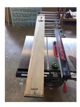
4. With the table saw blade raised to a tooth height above your material, the blade set 90° to the table and with the finish cut side against the fence, keep your material as flush as possible with the fence as you make your cut. See illustration:
