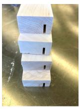
4. Now position one of your frame sides with the front face up and the groove to the left against the table saw blade. Raise the table saw blade so the highest tooth is about in the center of the groove you just cut.
